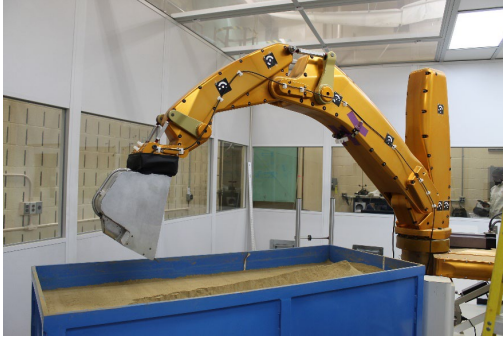
Figure 2. The Advanced Planetary Excavator (APEX) arm in the Excavation Lab at NASA Glenn Research Center. The Ultrasonic Bucket is attached as the end effector tool for the arm.
